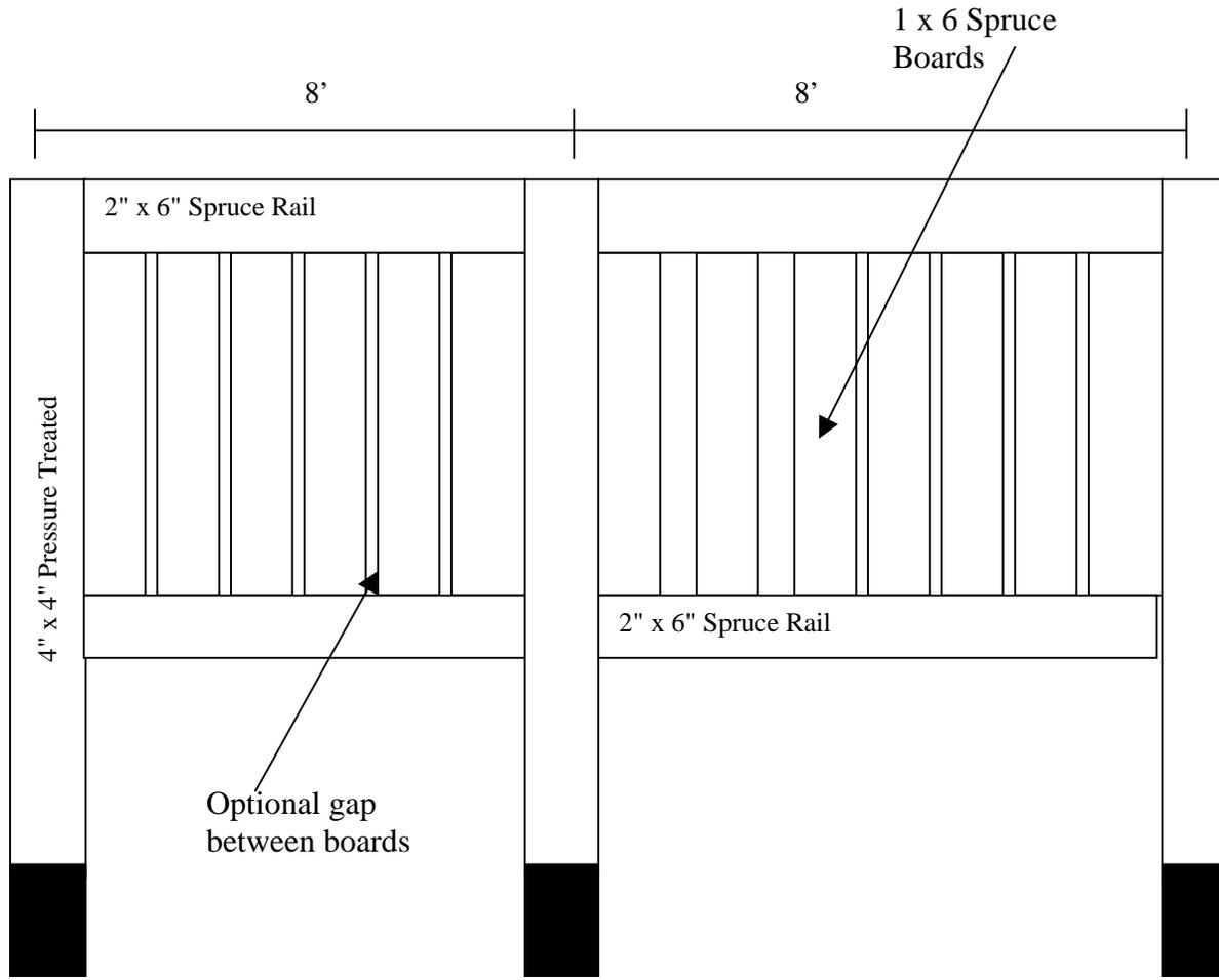
**10" Diameter x 3' Concrete Piles (Typical)
