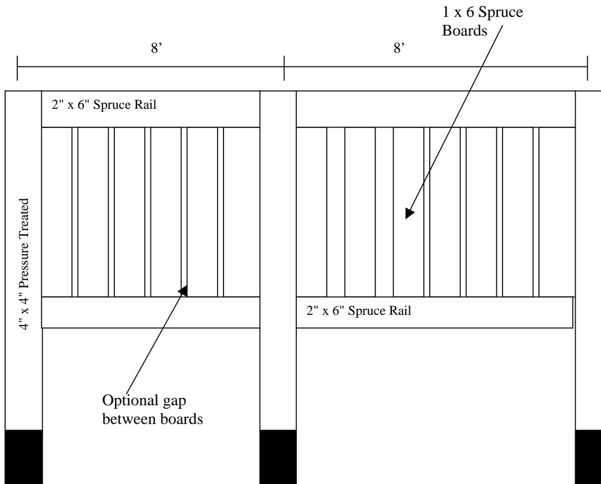
**10" Diameter x 3' Concrete Piles (Typical)
